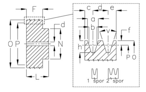
$\begin{array}{lll} d & = 10 \\ F & = 16 \\ L & = 28 \\ N & = 50 \\ Number of ribs = 1 \\ O & = 67.0 \\ P & = 63 \\ Type & = S \end{array}$
